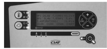
*Optimised <i>energy* management Information in multilingual clear text **AEROCONNECT™** is used to control the temperature or pressure, check the operating parameters, communicate with CIAT water chillers and diagnose and memorise faults.
