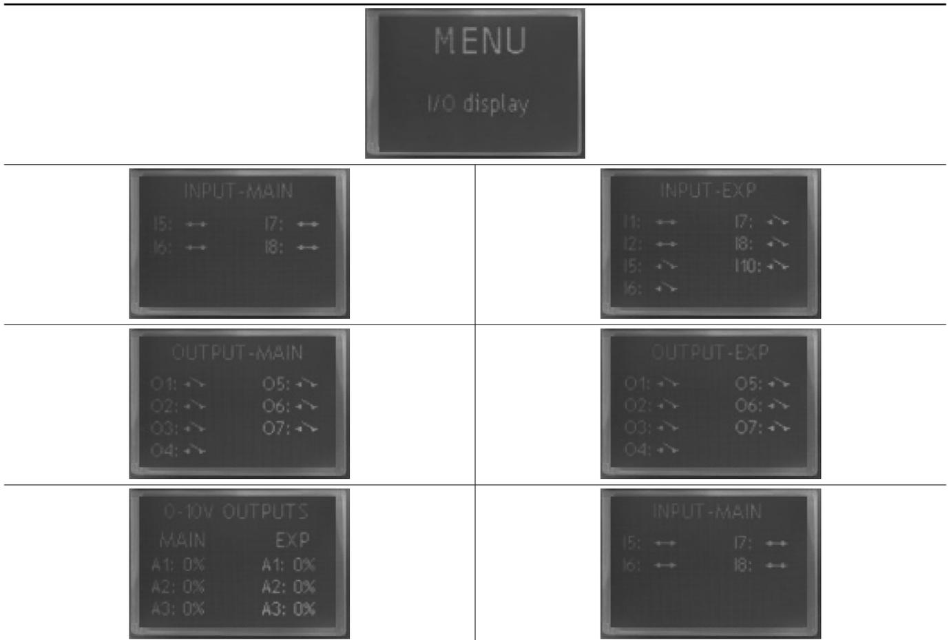
It is a section dedicated to reading the digital inputs and analog outputs of the controller of both the main and the expansion module (if installed; the expansion module is combined with some accessories)
