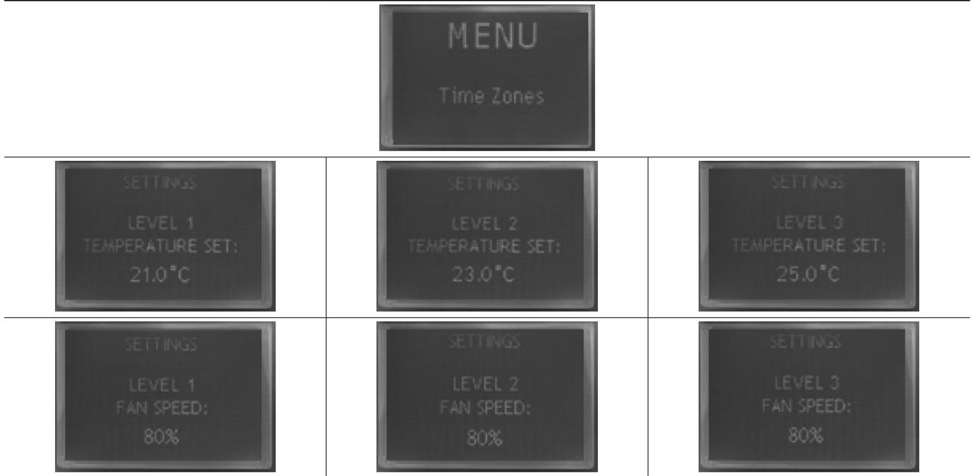
In the first 6 screens we have the possibility to set the 3 levels of both temperature and ventilation (in models without flow control) that you would like to alternate in the various time slots.
