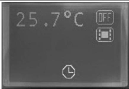
When the “clock” symbol appears, it means that the time bands function has been enabled. The function can be activated by the end user via a menu screen (for information on programming and enabling the time slots, refer to the next chapters). In this mode, the machine will switch on and off according to the programming carried out in the “time bands” menu. However, it will be possible to intervene on and off at any time via the display.
