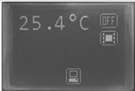
If under the OFF symbol appears the display symbol means that the machine is turned off by keyboard; this has priority over the turn on from BMS; you will have to turn on via display (see previous chapters), only then the command passes to the BMS system.
