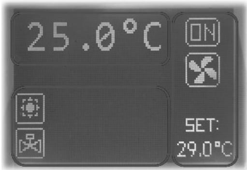
For a better understanding we will divide the main screen into two boxes (which will be referred to as left box and right box in the following) divided by a vertical dividing line (not actually present in the display).
