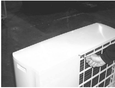
remove the middle screw (rear section)
