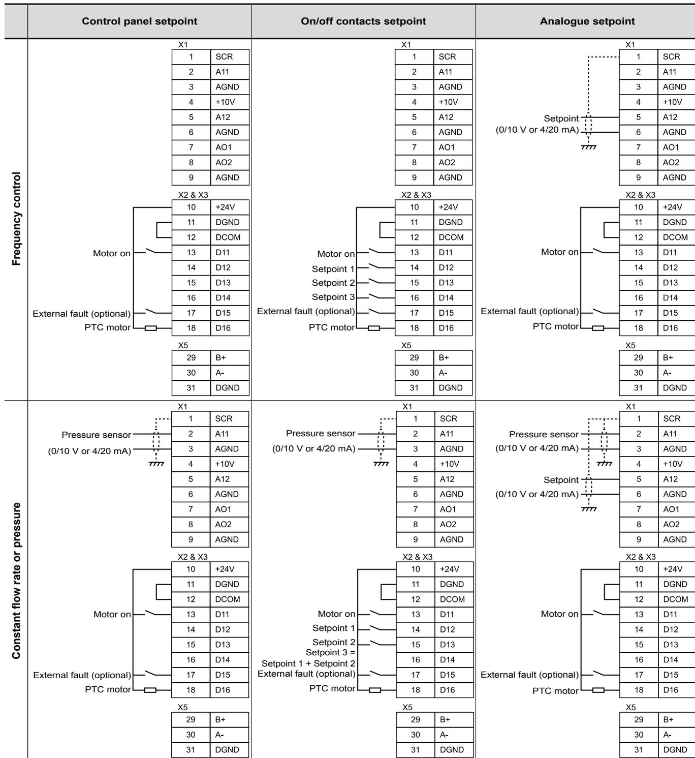
(\*) For control cables, use a paired twisted cable. If the cable is longer than 10 metres, (with a maximum of 30 metres for a 0/10V signal, and 300 metres for a 4/20mA signal) use a shielded twisted pair cable, with the shielding connected to earth at least one end (ideally, it should be connected to earth at both ends).
