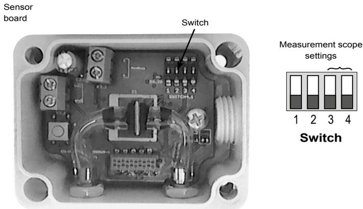
To configure your device, switch it off and enter the desired settings using the switches as shown in the tables. Once configured, switch the sensor back on.
