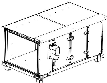
External unit: assemble the protection cap provided for this purpose, supplied as a kit (optional), as shown below. Protecting the inverter against weather and UV is mandatory.
